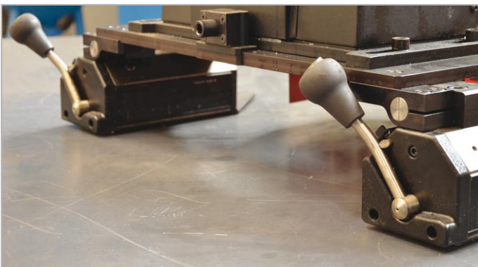
Permanent magnets need no power supply from the mains. A self-locking device prevents any possible accidental movement of the handle and deactivation of the magnet.
