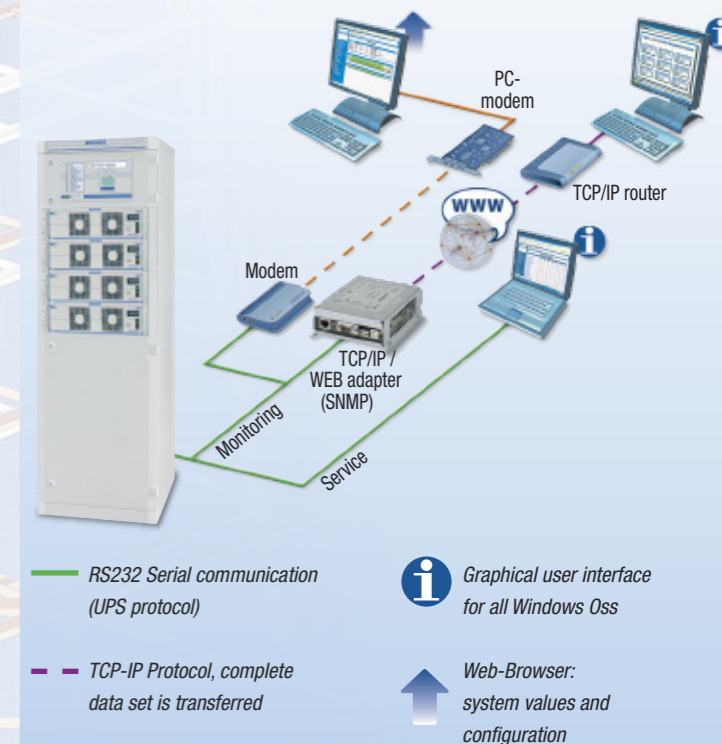
Fig. 10: Monitoring concept of the MCU 2500
