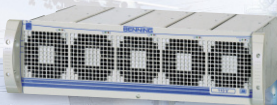
Fig. 3: 19" modular rectifier shelf with 5 modules TEBECHOP 3000 HDI output voltage 110 V, output current 100 A
