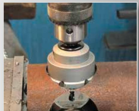
Bohren in Rohre
