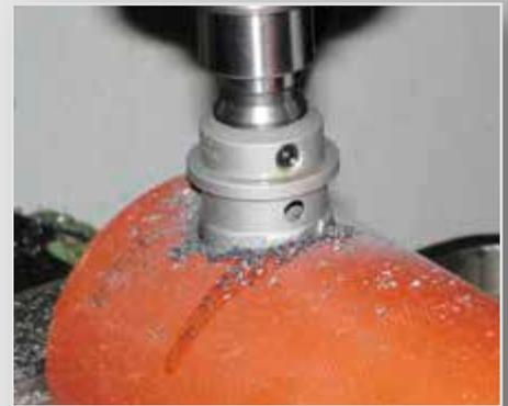
Bohren in Rohre
