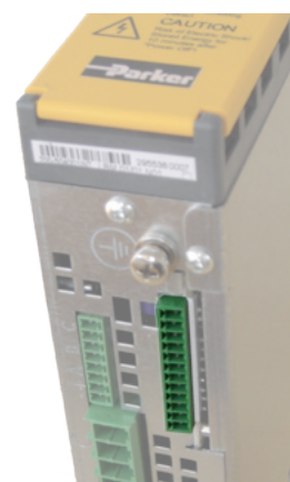
Hiperface DSL connection On the bottom, near power connections
