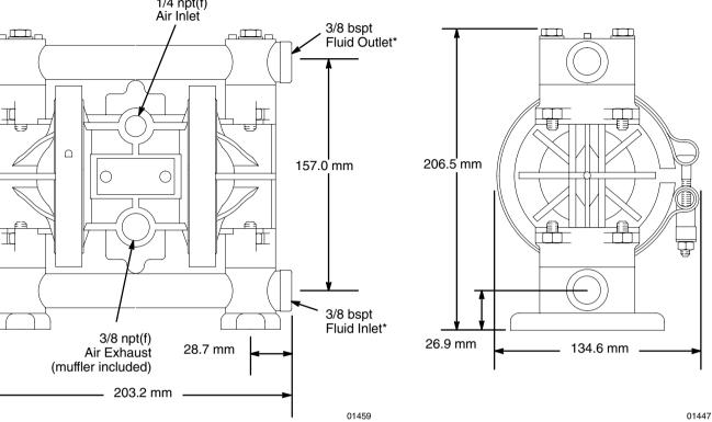
\* Pumps 810.0465-810.0474 have npt(f) threads on the fluid inlet and fluid outlet.
