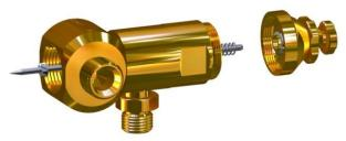
4. Unscrew sealing cap [80] by hand.
