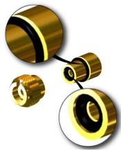
10. Dismantle sealing screw [150] by hand; check the two O-rings [151 + 152] of the sealing screw for any damages and replace them, if necessary.
