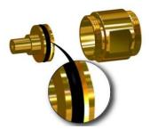
8. Press piston [140] out of the cylinder by hand. Check the O-ring [141] of the piston for any damages and replace it, if necessary.
