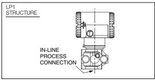
Figure 7. Low Profile Structure - LP1 Shown
