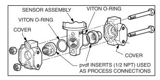
Figure 1. Bottomworks Shown with 1/2 NPT pvdf Inserts
