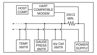
Figure 21. Typical Multidrop Block Diagram
