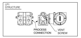
Figure 11. Horizontal Mounting with Vent Screw
