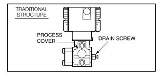
Figure 4. Vertical Mounting - Cavity Draining
