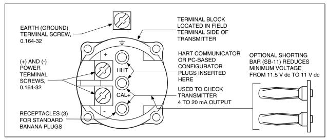
Figure 23. Field Terminal Block
