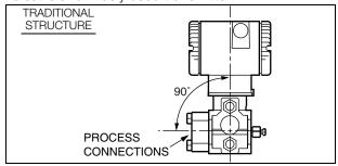
Figure 3. Vertical Mounting Showing Process Connections at 90 degrees
