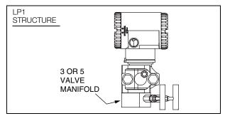
Figure 8. LP1 Shown Directly Mounted to Manifold
