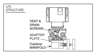
Figure 15. Adapter Mount to Existing Coplanar Manifold
