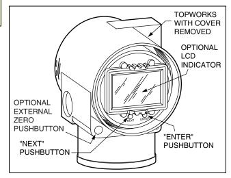
Figure 22. LCD Indicator with On-Board Pushbuttons
