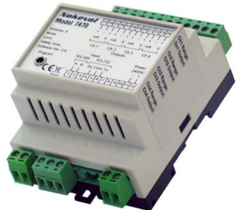
The transmitter 7470 provides an economical means of converting digital data to analog signals, mA / V, and transmitting them to four field instruments. Configuration is simple by MekuWin program or the general purpose hand held programmer 6790. The transmitter uses the simple Nokeval SCL protocol. One serial data bus accepts 31 7470 transmitters or other serial instruments, that is 124 output channels. Typical applications are PC-based programs or PLC.
