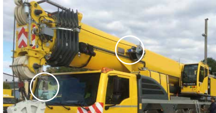
An all-terrain telescopic crane fitted with a Motec camera and monitor system.
