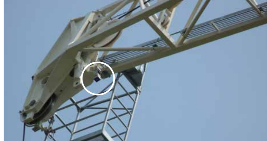
Motor zoom camera at a jib. The pendulum mounting allows the camera to adapt to the jib's tilt angle.
